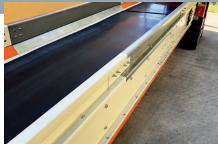
Non-magnetic section in stainless steel AISI 304
