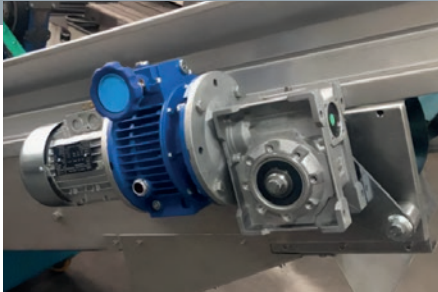
Gear motor with mechanical variator
