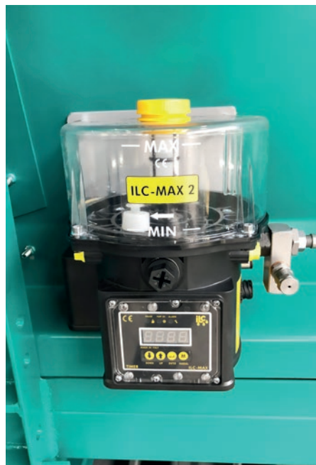
Hydraulic lubrication control unit
